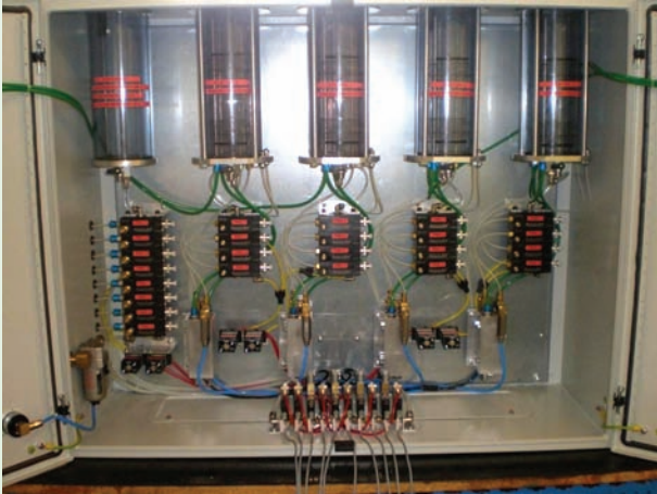
8 pumps for outside lubrication 8 pumps for inside lubrication 8 pumps for additional lubrication
