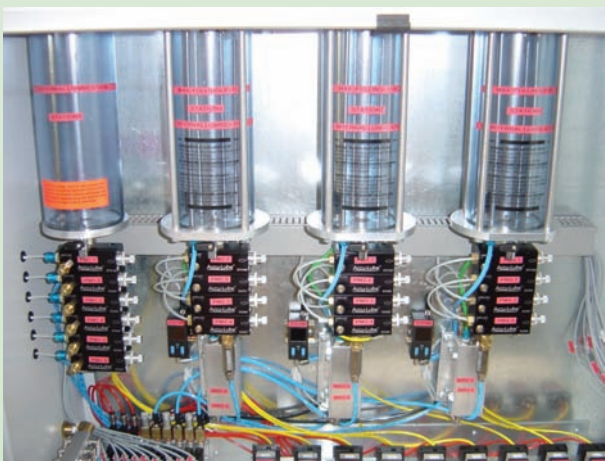
6 pumps for outside lubrication 6 pumps for inside lubrication 6 pumps for additional lubrication
